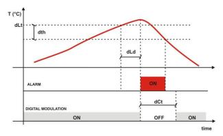
Until alarm delay time (dLd) is active the total compressor capacity will be limited to Cdd.
